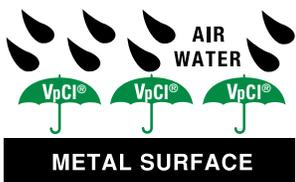
*BullFrog VpCIs bond with metal surfaces to form a protective 'Molecular Umbrella,' sealing out air and moisture that cause rust and corrosion.*
