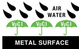
Bull Frog® VpCI™s bond electrochemically with metal surfaces to form a protective “Molecular Umbrella”, sealing out the air and moisture that cause rust and corrosion.
